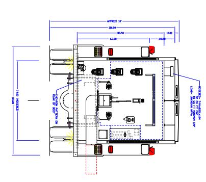
6. THE EFFECTIVE DOOR OPENINGS WILL BE APPROX. 2" LESS THAN THE NOTED COMPARTMENT OPENING FOR ROLL UP DOORS AND UP TO APPROX. 4" LESS FOR HINGED DOORS
